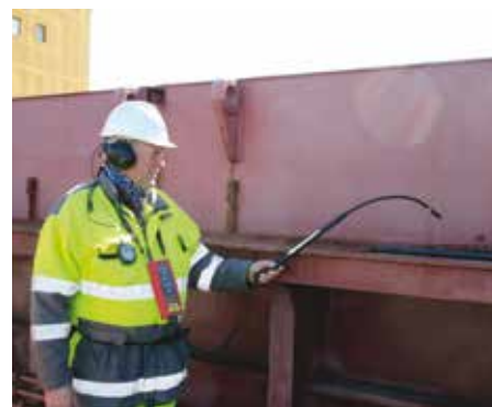
Testing for leaks by ULD
