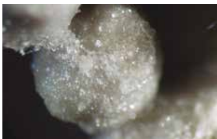
Crystal bridges between fertilizer particles cause caking
