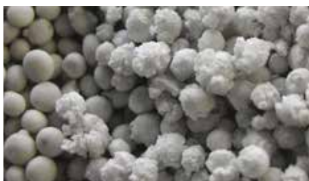
Disintegrated fertilizer due to water absorption
