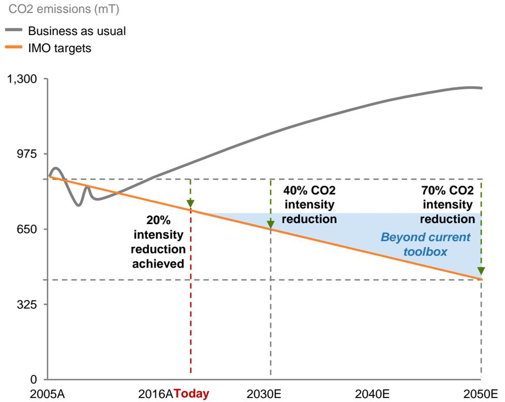
The industry's current toolbox can reduce emissions by 20-25% – clean fuel alternatives will be required to meet IMO's targets
