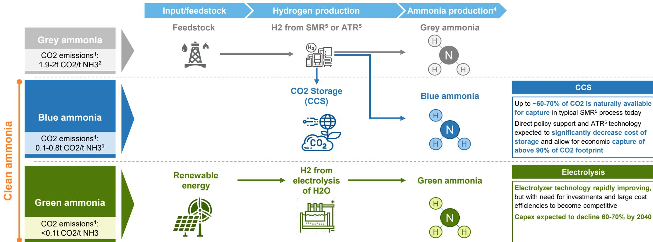
The Haber-Bosch process is used to synthesize ammonia from hydrogen<sup>1</sup>, producing an identical ammonia molecule regardless of “color”
